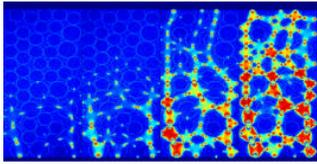
Photoelastic measurement of stress propagation from sinusoidal compression of a densely packed unbonded granular material under constant pressure. (Mark Shattuck)
